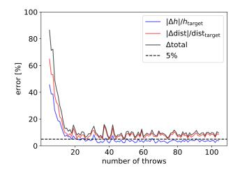
**Figure 3.** Evolution of the mean  $\Delta h$  (blue),  $\Delta dist$  (red) and  $\Delta total$  (black) with the total number of throws in 100 experiments. The dotted line represents the target error range of 5%. In general, the error of all three quantities decreases as the number of throws increases, which indicates the success of the machine to provide meaningful recommendations.
